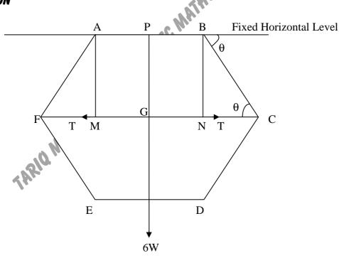
Since W be weight of each rod therefore weight of six rod is 6W which acts at the centre of gravity G of hexagon. Let L be the length of each rod and  $\theta$  be the angle which rod BC makes with horizontal. Let AM and BN are perpendicular on CF. Let P be the midpoint of the AB. Let T be the thrust in the rod FC.
