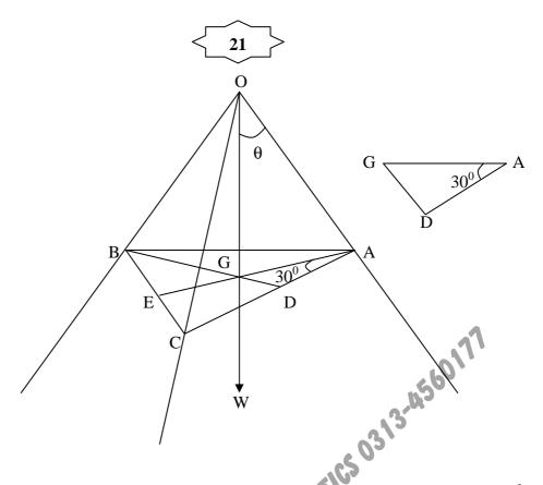
Since the length of each rod is *l*. Therefore  $OA = OB = OC = AB = BC = CA = \frac{l}{2}$  The vertical line through O meets the plane of  $\triangle ABC$  at point G. Where G is the point of intersection of the medians AE and BD. Let each rod makes an angle  $\theta$  with OG. Let T be the tension in each string. Then
