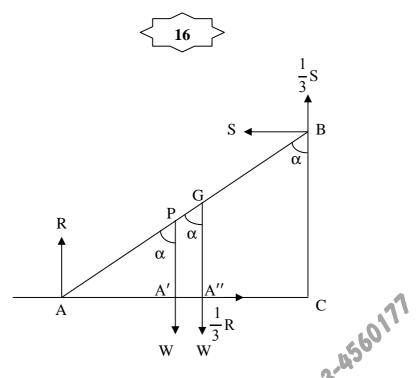
Let AB be a ladder of length 2L makes an angle of  $\alpha$  with vertical. W is its weight acting downward from its midpoint G. R and S are normal reactions of ground and wall respectively.  $\frac{1}{3}$ R and  $\frac{1}{3}$ S are forces of friction of ground and wall respectively. Let P be the LT. MOOD GADRI M.SC MATH point where weight W is attached. Since AB = 2L Therefore AG = BG = L. Let AP = xNow we have to prove that
