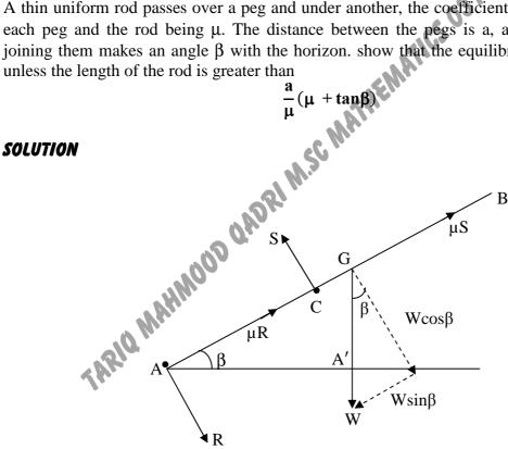
Let AB be a rod of length 2L makes an angle of  $\beta$  with horizon. W is its weight acting downward from its midpoint G. R and S are normal reactions of pegs at A and C respectively.  $\mu$ R and  $\mu$ S are forces of friction.
