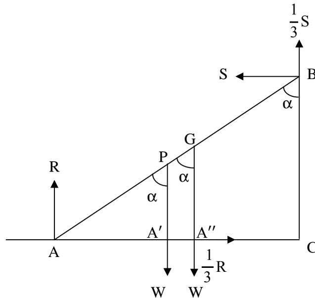
Let AB be a ladder of length  $2L$  makes an angle of  $\alpha$  with vertical.  $W$  is its weight acting downward from its midpoint  $G$ .  $R$  and  $S$  are normal reactions of ground and wall respectively.  $\frac{1}{3}R$  and  $\frac{1}{3}S$  are forces of friction of ground and wall respectively. Let  $P$  be the point where weight  $W$  is attached. Since  $AB = 2L$  Therefore  $AG = BG = L$ . Let  $AP = x$
