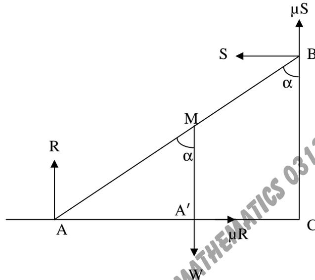
Let AB be a light ladder which makes angle  $\alpha$  with vertical. Let M be the position of the man of weight W when the ladder is in limiting equilibrium. R and S are normal reactions of ground and wall respectively,  $\mu R$  and  $\mu R$  are forces of friction of ground and wall respectively.
