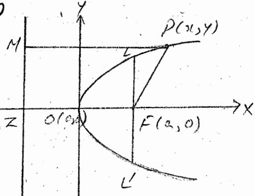
through the focus and perpendicular to the directrix is called axis of the parabola. The point where the parabola meets its axis is called the vertex of the parabola.
