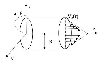
The velocity component in the radial and tangential direction are zero.  $V_r = V_{\theta} = 0$ . Under these assumptions the equation of continuity in cylindrical coordinates is
