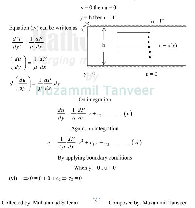
$$\Rightarrow u = \frac{1}{2\mu} \frac{dP}{dx} \cdot y^2 + c_1 y \dots (vii)$$
