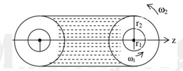
Assume the flow between the cylinders to be peripheral (circular or round about) so that we have only the tangential component of velocity  $V_{\theta}$  i.e.  $V_r = V_z = 0$ . The equation of continuity in cylindrical coordinates is
