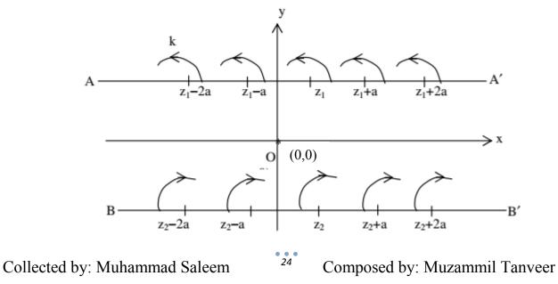
Let one vortex on infinite row AA' be at  $z = z_1$  and one vortex on infinite row BB' be at  $z = z_2$ , so that the system consists of vortices K at  $z = z_1 \pm na$  and vortices '-K' at  $z = z_2 \pm na$ , n = 1, 2, ...
