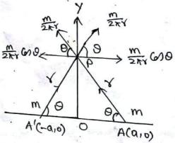
velocity at p due to A' along  $A'p = \frac{m}{2\pi r}$ components of velocities L to y-anis' at pare equal in magnitude but opposite in direction
