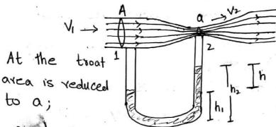
and a monometer tube is attached. Let the monometer liquid have a density \$2. Let vi and v2 be the flow speed at pt 12 and 2. Now by applying Bernoulli's eq; we have;
