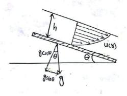
since the flow over the plate is parallel and occurring in the xi-direction only; so V=w=0
