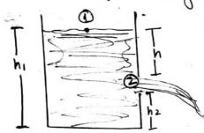
through which a liquid is being discharged into the open atmosphere. Let vi be velocity at top surface and vi be velocity at orifice. Then by using Bernoulli's eq; we have
