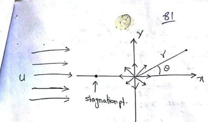
11 is clear that at some pt along the -ive n-anis the velocity due to the source will just cancel the velocity due to the uniform stream; and a stagnation pt will be exeated.
