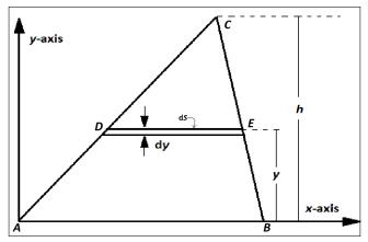
Moment of inertia of typical elementary strip about side AB (x-axis) is given by
