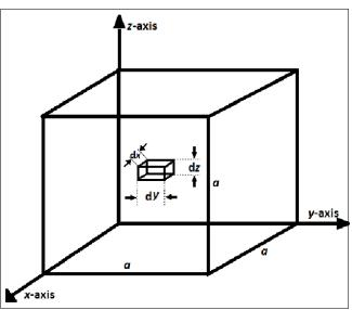
**Example 8:** Calculate the inertia matrix of a (uniform solid) cube of mass M at one of its corners, by taking coordinate axes along its edges. **Solution:** Repeat example 7 for a = b = c and get
