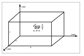
of mass dm, volume dV and dimensions dx, dy and dz, is shown in the figure.
