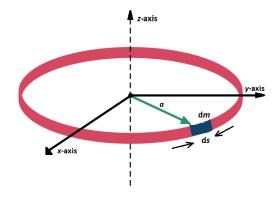
Moment of inertia of typical element about z-axis is given by
