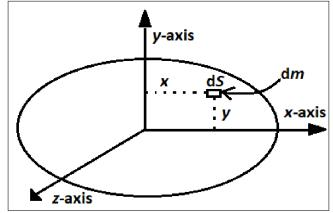
Let M and  $\sigma$ , respectively, be the mass and surface (areal) mass density of the elliptical plate. To find moment of inertia about major axis (x-axis), we proceed as follows. We divide plate into large number of elementary rectangular pieces of infinitesimal area with sides parallel to x and y axis. One typical area element having mass dm, area dS, length dx and width dy is shown in the figure at point (x, y).
