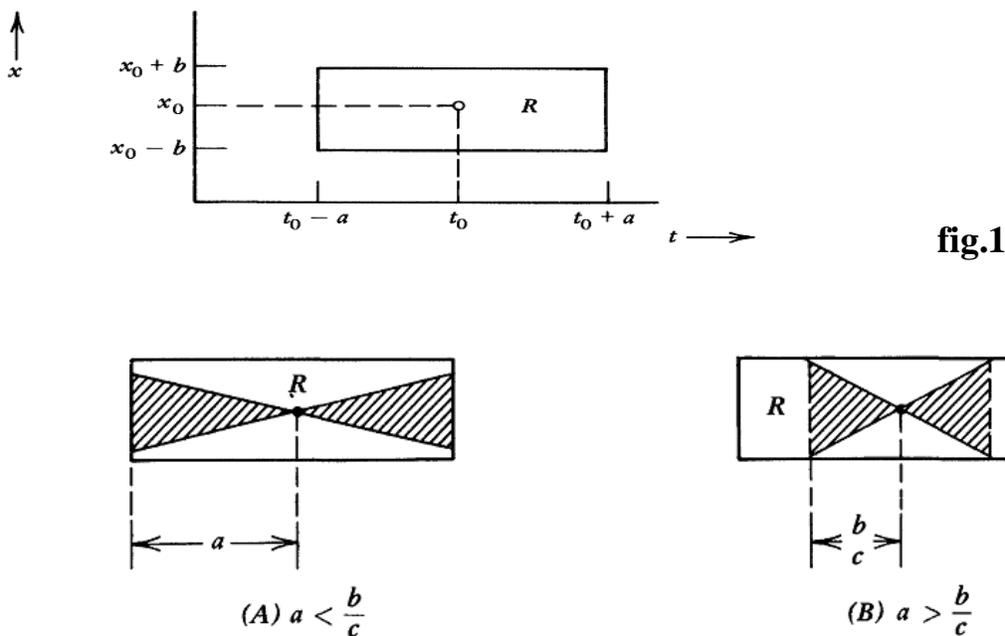
**Fig. 54.** Geometric illustration of inequality (2) for (A) relatively small  $c$ , (B) relatively large  $c$ . The solution curve must remain in the shaded region bounded by straight lines with slopes  $\pm c$ .
