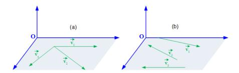
Figure 2.11: (a) Coplanar and Concurrent (b) Coplanar and Non-Concurrent vectors
