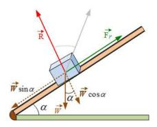
Figure 5.4: Angle of friction
