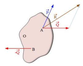
Figure 3.57: Resultant of P and Q at A.
