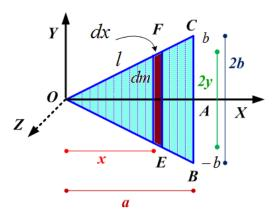
Figure 11.43: Uniform triangular disc
