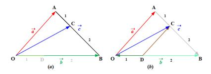
Figure 2.35: Vector addition by head to tail rule.
