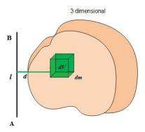
Figure 11.5: Moment of inertia of 3 dimensional system
