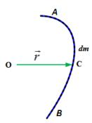
Figure 10.7: Center of mass of 1 dimensional system
