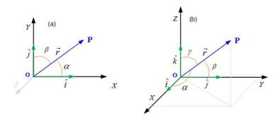
Figure 2.14: Direction angles of  $\vec{r}$ .
