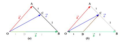
Figure 3.26: Vector addition by head to tail rule.
