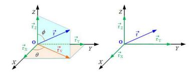
Figure 2.18: Orthogonal components of a vector in 3 space.
