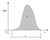
Figure 6.2: Impulse of a force
