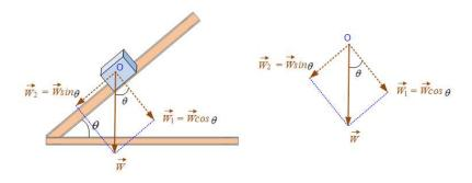
Figure 2.15: Orthogonal components of a vector.
