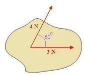
Figure 3.17: Two concurrent forces acting on a body.
