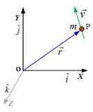
Figure 7.2: Angular momentum about origin in a plane
