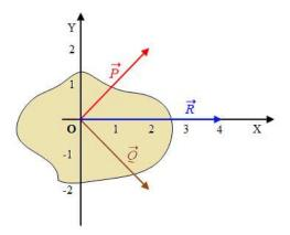
Figure 3.33: Resolved components of a force
