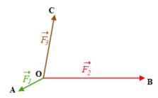
Figure 3.40: Three concurrent and non-coplanar vectors
