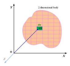
Figure 10.9: Center of mass of 2 dimensional system
