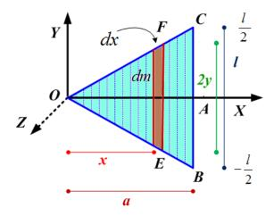
Figure 11.44: Uniform equilateral triangular disc
