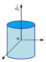
Figure 11.19: Principal axis for cylinder
