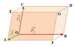
Figure 3.41: Three concurrent and non-coplanar vectors
