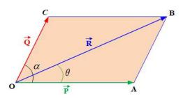
Figure 3.11: Parallelogram of vectors
