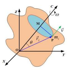
Figure 11.15: Angular momentum of a rigid body
