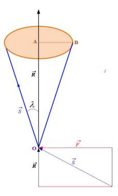
Figure 5.3: Cone of friction
