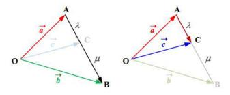
Figure 3.24: Vector addition by head to tail rule.
