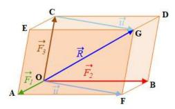
Figure 3.42: Addition of three concurrent and non-coplanar vectors
