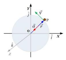
Figure 7.3: Angular momentum in uniform circular motion.
