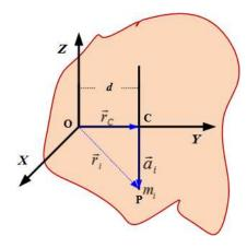
Figure 11.10: Parallel axis theorem
