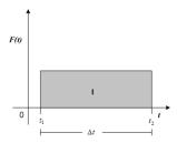
Figure 6.1: Impulse of a force
