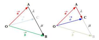
Figure 2.33: Vector addition by head to tail rule.
