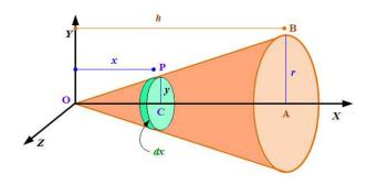
Figure 11.58: uniform solid right circular cone
