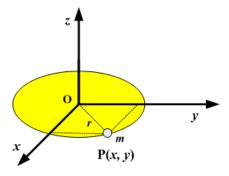
Figure 11.11: M.I. about perpendicular axis
