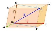
Figure 2.42: Addition of three concurrent and non-coplanar vectors
