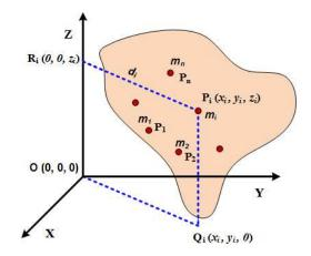
Figure 11.9: M.I of of a system of particles
