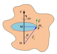
Figure 11.14: Angular momentum of a body
