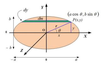
Figure 11.51: Uniform elliptic disc
