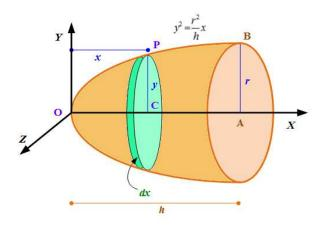
Figure 11.59: solid paraboloid
