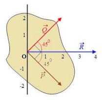
Figure 3.32: Resolved components of a force
