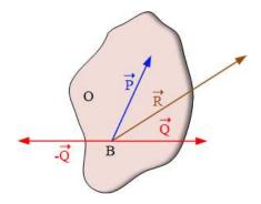
Figure 3.58: Resultant of P and Q at B.
