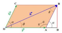
Figure 2.25: Parallelogram of vectors
