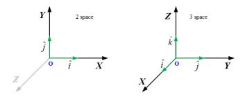
Figure 2.6: Unit vectors along coordinate axes
