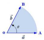
Figure 2.13: angle between two vectors.
